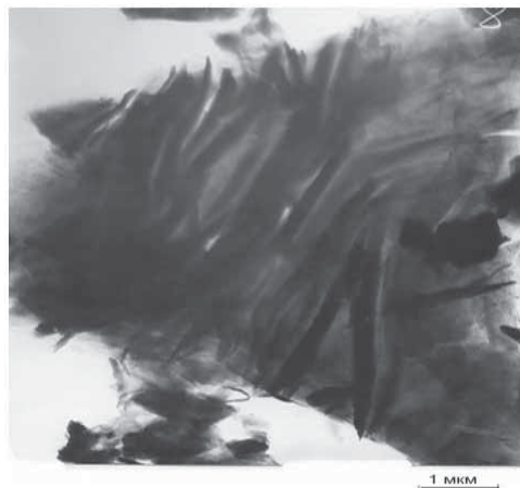
Fig. 4. Electron micrograph of a sample of traditionally baked vermiculite.
