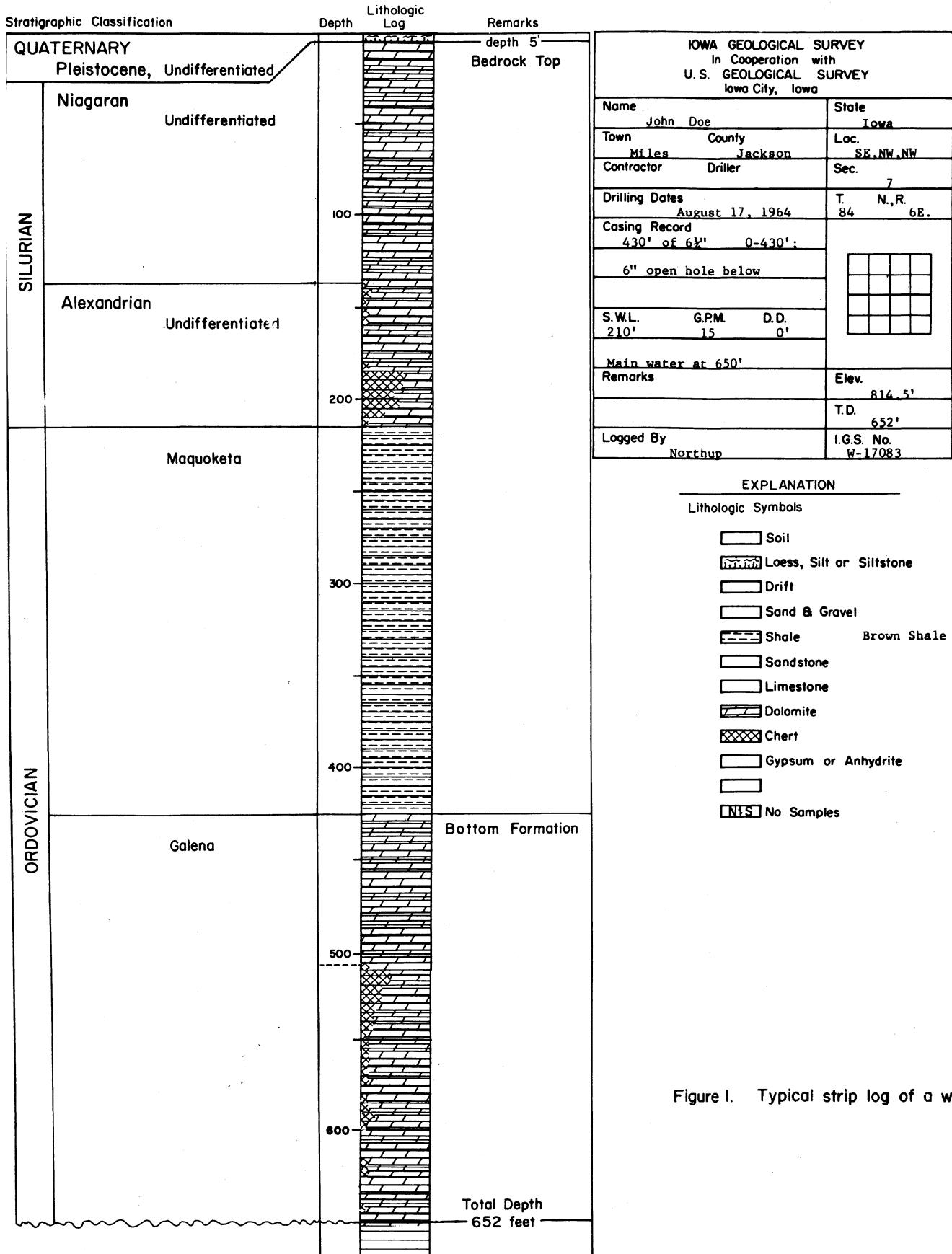
Figure I. Typical strip log of a well.
