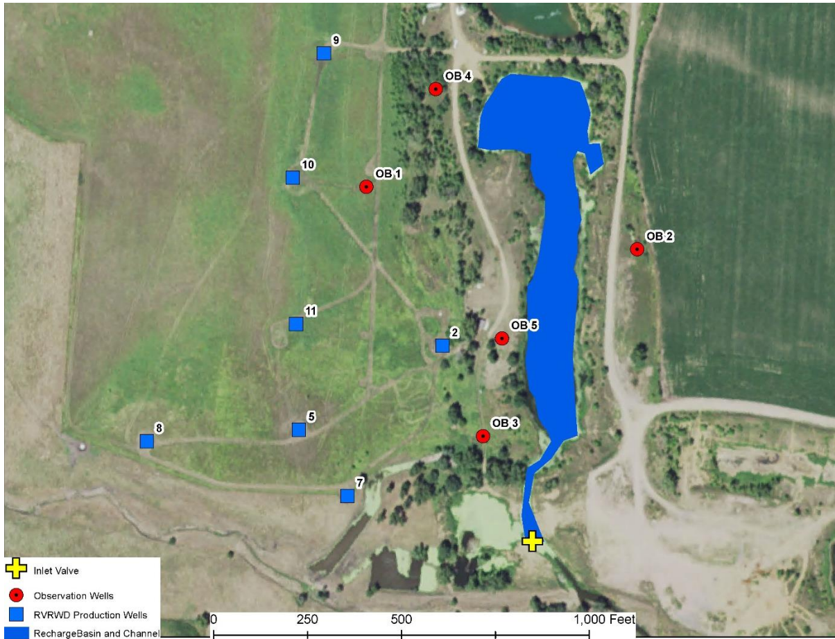
Figure 2. Sand and gravel quarry location used as a recharge basin. Unnamed Creek was re-routed into the quarry.
