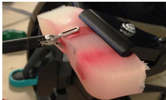
Figure 3.10: The artificial tissue with tumors implemented at different depth
