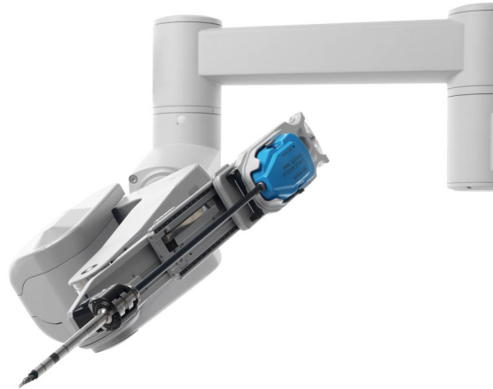
Figure 1.3: The EndoWrist ® instrument as the end-effector of da Vinci surgical system (©Intuitive Surgical Inc.) [2].
