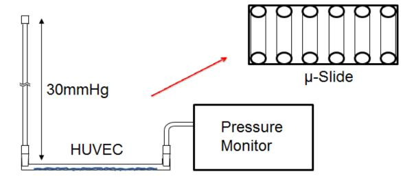
Figure 2.1 The experimental setup for the elevation of hydrostatic pressure
