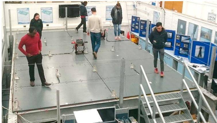
Fig. 4. Modal test of the floor structure occupied by six walking people.
