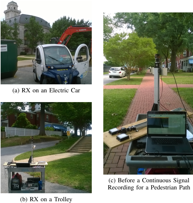
Fig. 3. Photos of the measurement setup. The TX was installed on a clock tower at a height of 90 feet (27.4 m) to emulate a microcell deployment. Either an electric car or a two-layer trolley was used to transport the RX. For both cases, the platform for the RX could be rotated horizontally and tilted with composite wood shims to align the beam.
