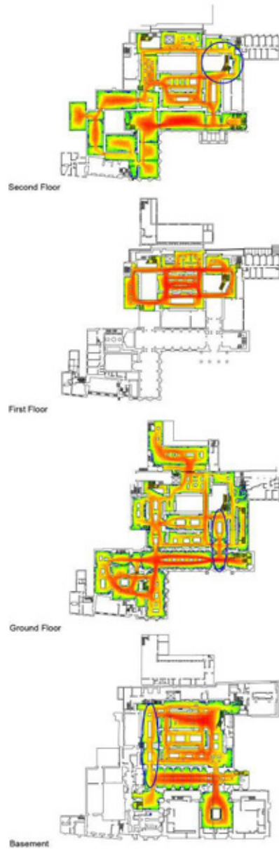
Figure 8 - Agent-based models for the Ashmolean Museum. Red areas show high movement rates and blue ones low. The circles signify the areas where differences are observed with real movement. 50 agents are released with standard properties (Turner and Penn, 2002): a walking pace of about 1.5ms -1 , three steps to decision and a field of view of 170°.
