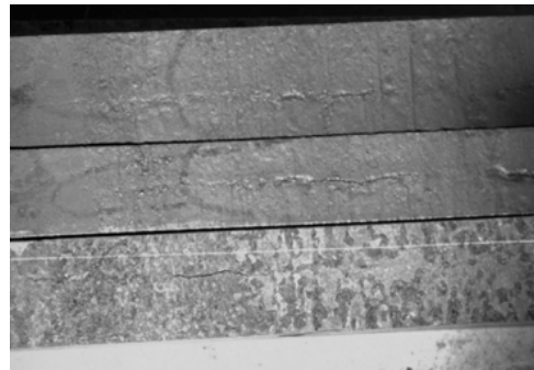
Figure 9. Defective steel samples placed on a carriage for imaging with the HTP-C instrument.
