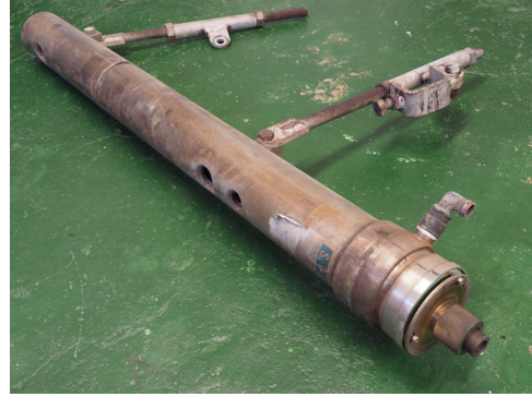
Figure 5. HTP-C cooled housing with apertures for two cameras and a laser stripe projector. The exterior shows extensive marking after being suspended above the caster for a period of several weeks.
