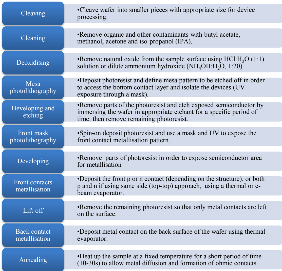
Figure 3.13. Flow chart of standard device fabrication process for TPV test cells.
