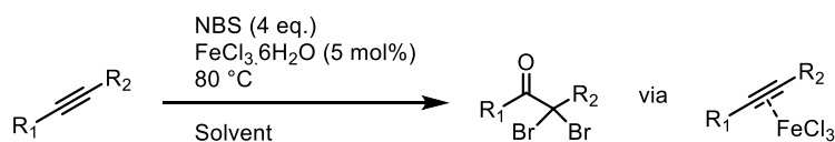
Scheme 2.26 Dibromohydration of alkynes via the generation of hypobromous acid with an iron catalyst in a solvent mixture of THF/ \text{H}_2\text{O} 171,172 or MeOH 170
