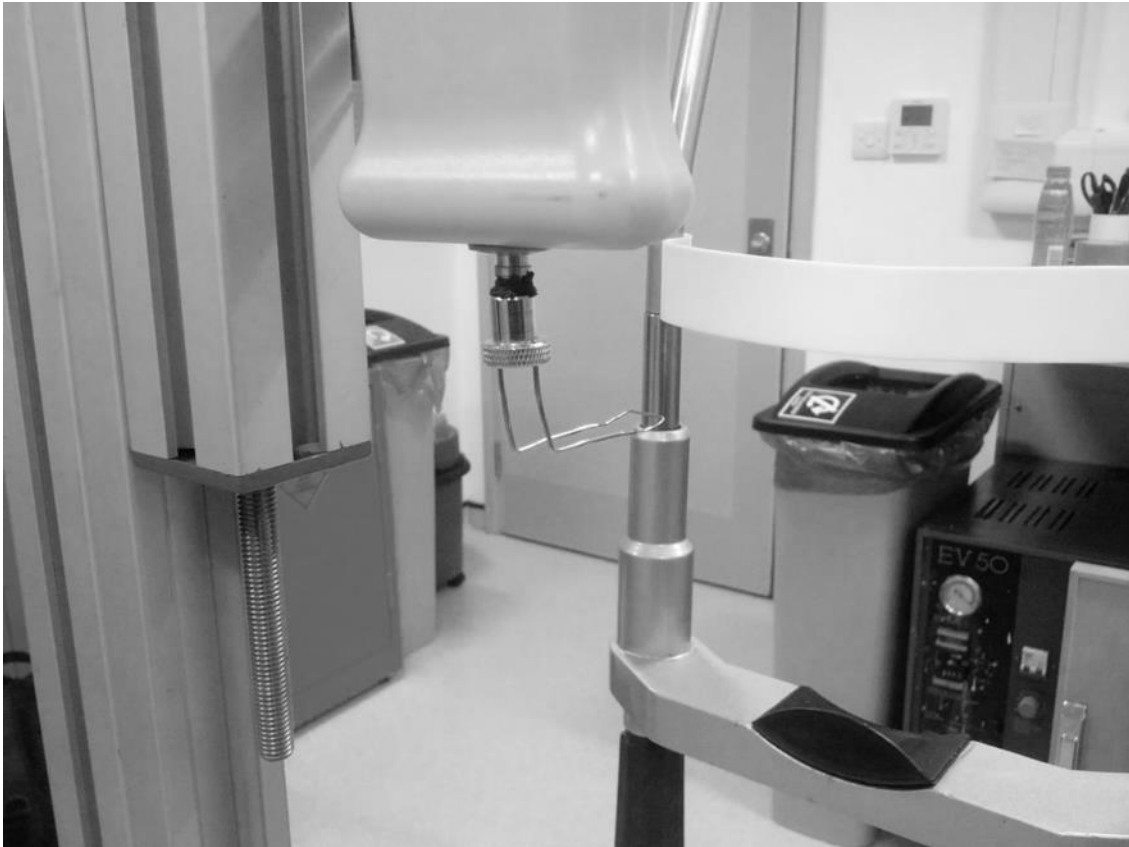
Figure 35. | Eyelid attachment that connects to the DFG and produces direct force measurement in Newtons.
