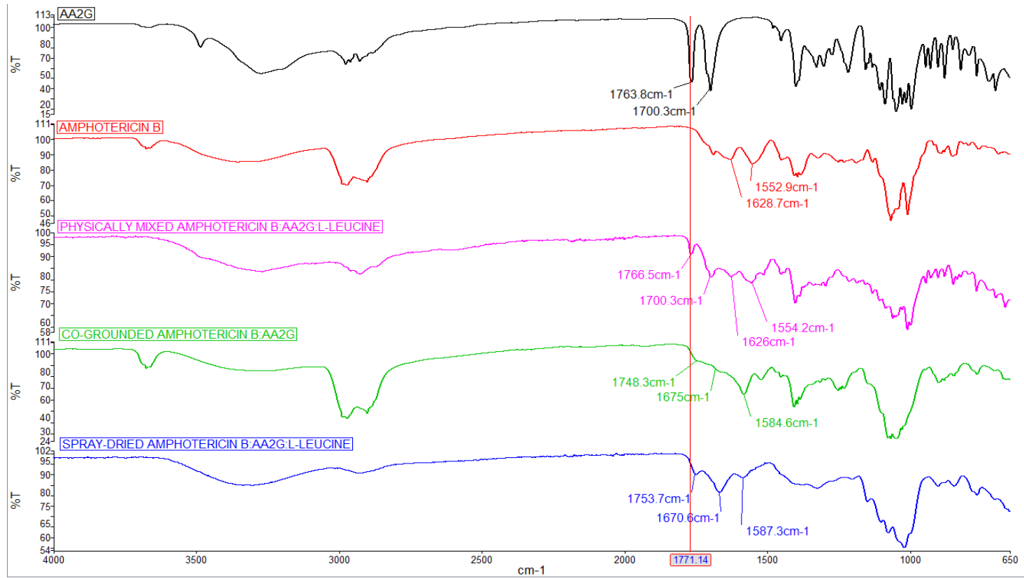
Figure 3.33: FT-IR spectrum of spray dried and physically mixed amphotericin B: AA2g: L-leucine (split view)
