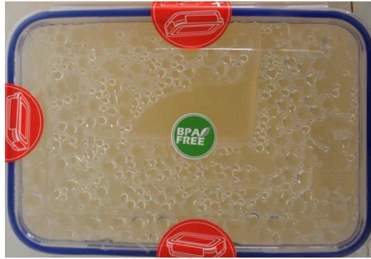
Figure 3.11: Photograph of the gelatine phantom, which is essentially a food container containing two smaller plastic containers inside.
