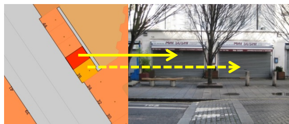
Figure 2: A capture example. The yellow polygon (with the yellow dotted line) is the 'addressable polygon' for this hereditament (a restaurant). The SMV shows that it requires 77m^2 (GEA) but the yellow polygon only offers 41m^2 . The red polygon next door, which has no OSAB 'address' on the relevant floor, offers 37m^2 , which provides a combined floor area of 78m^2 . The software accepts this as an optimal match. (Data: © Crown Copyright/database right 2012. An Ordnance Survey / EDINA supplied service.)
