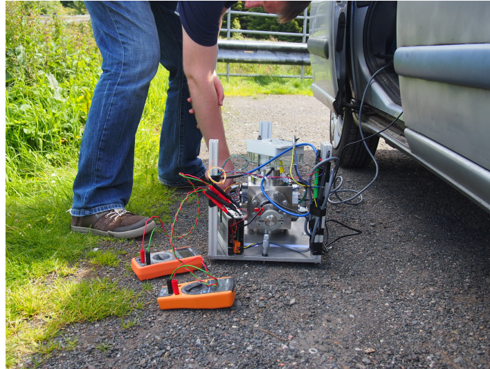
Figure 7. An image of the gravity measurement being conducted at the top of the hill. The user can be seen levelling the platform before the data is recorded.
