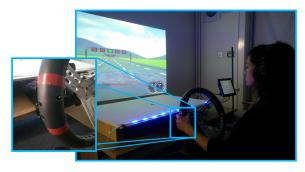
Figure 1: Multimodal feedback for mid-air gestures in a simulated driving scenario. Feedback types are 1) visual, 2) auditory, 3) ambient lights, and 4) cutaneous push.
