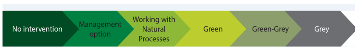
Figure 3.2 Continuum of scheme scale decisions from no intervention through to a grey engineering solution, commonly used in flood risk management (after Roca et al., 2017).
