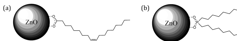
Figure 2. Diagram illustrating ZnO NPs capped with (a) OA and (b) DOPA.
