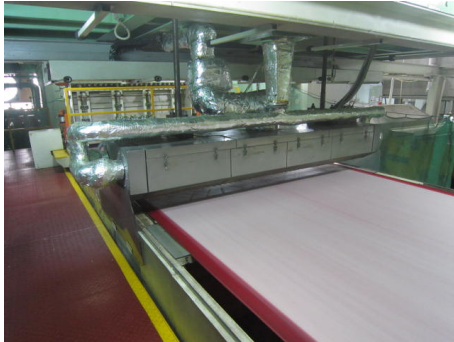
Figure 1.7: Compound for non-woven fabric production line. Source: product catalogue Zhejiang Sanlong Universal Machinery Co., Ltd 23 .
