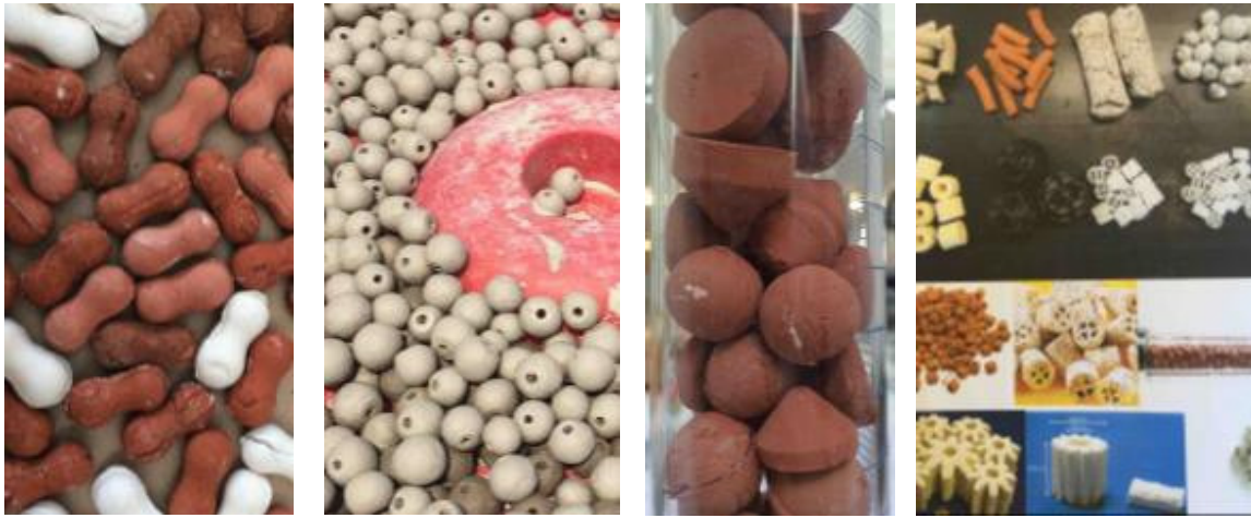
Figures 4-7 Ceramic filter modular units & geometries ideas for geometry
