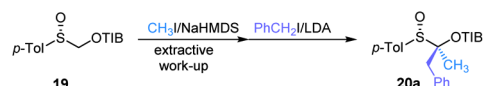
Figure 9. (A) Synthesis of disubstituted \alpha -sulfinyl benzoates through alkylation of monosubstituted derivatives. (B) Proposed model rationalizing diastereoselectivity. (C) Sequential alkylation of \alpha -sulfinyl benzoate 19 . a Reaction conditions: benzoate 14 (1.0 equiv), R 2 X (1.5 equiv), LDA (1.8 equiv), THF, -78 °C; then 0 °C. b Determined by 1 H NMR analysis. c Benzoate 19 (1.0 equiv), CH 3 I (1.1 equiv), NaHMDS (1.1 equiv), -78 °C to rt; extractive workup; PhCH 2 I (1.5 equiv), LDA (1.8 equiv), THF, -78 °C then 0 °C.
