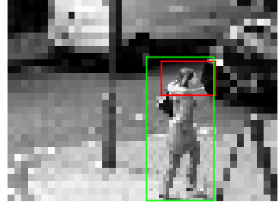
Fig. 3. A person being tracked and sampled at multiple resolutions. The green rectangle represents a prior model of shape and scale, differences under which should be created by something with human proportions. The red rectangle is the expected position of the head within the shape model.
