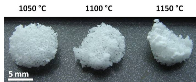
Figure 2. Biosilicate ® scaffolds produced by the replica method using the standard slurry concentration of 40 wt.% and respective sintering temperatures employed. The scaffolds were infiltrated twice and sintered for 1 h at the selected temperatures. (Some samples were damaged during handling or were partially fractured to observe their interior region.)
