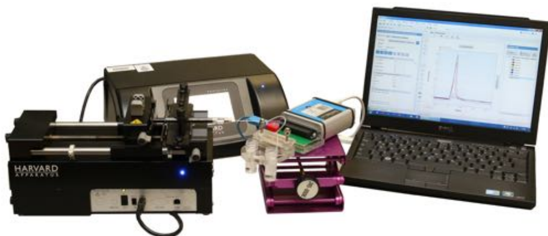
Figure 5.10: Photograph of the whole measurement setup illustrating a 8-channel microfluidic chip fastened into the chip holder, connected to the syringe pump and potentiostat.
