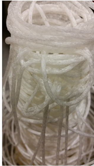
Figure 3.6: Fibres produced from the larger single-screw melt-compounder. The fibres were brittle, had air pockets within, and very rough surfaces.
