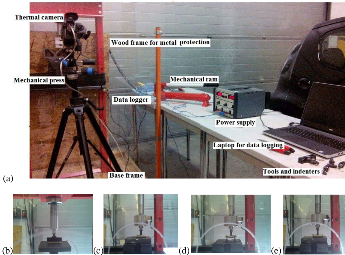
Figure 2: (a) Experimental setup for mechanical loading tests, (b) Flat plate, (c) Circular punch, (d) three-point bend (e) Rod test
