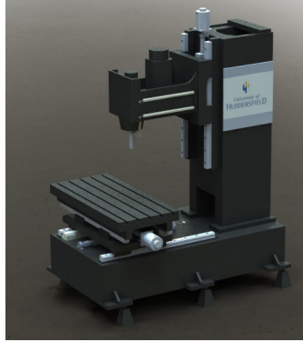
Figure 1: Three-axis C-Frame machine tool.
