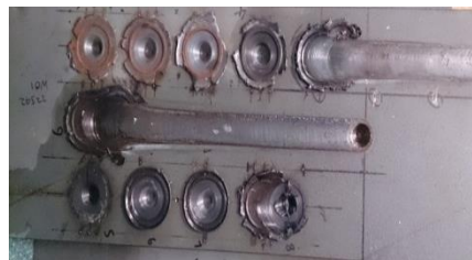
Figure 1: EH46 steel plate showing the position of the seven plunge trials.
