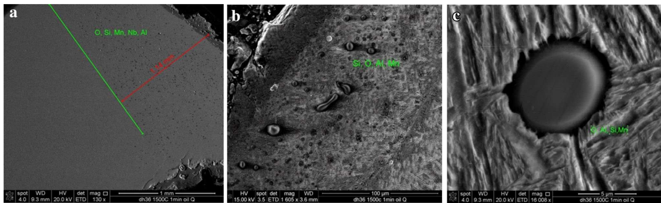
Fig. 9 Heat treatment with 1500 °C and cooling rate 30 °C/s, soaking time 1 min. Segregation is forming with less soaking time when temperature approaches the melting point of base metal
