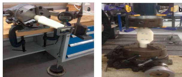
Figure 2. (a) Cantilever test setup. (b) Tensile test setup.
