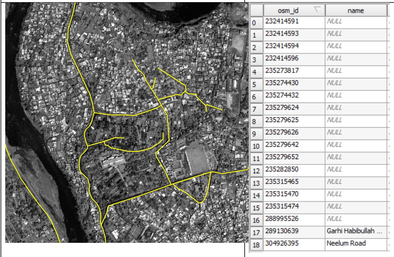
Figure 3.4 Primary and secondary roads for Van are shown in yellow overlaid on a high resolution image. The attribute table in the side show that the data are well populated.
