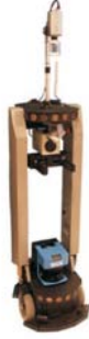
Fig. 2. ActivMedia Peoplebot. It is equipped with a SICK LMS 200 laser scanner and panoramic camera (NetVision360 from Remote Reality).
