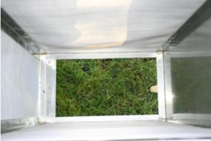
Figure 2 - View from above modified Gerking box sampler with cutting blade retracted to show size of sample obtainable.
