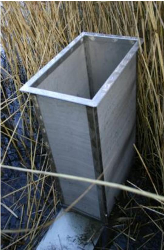
Figure 3- Modified Gerking box sampler within reed bed.
