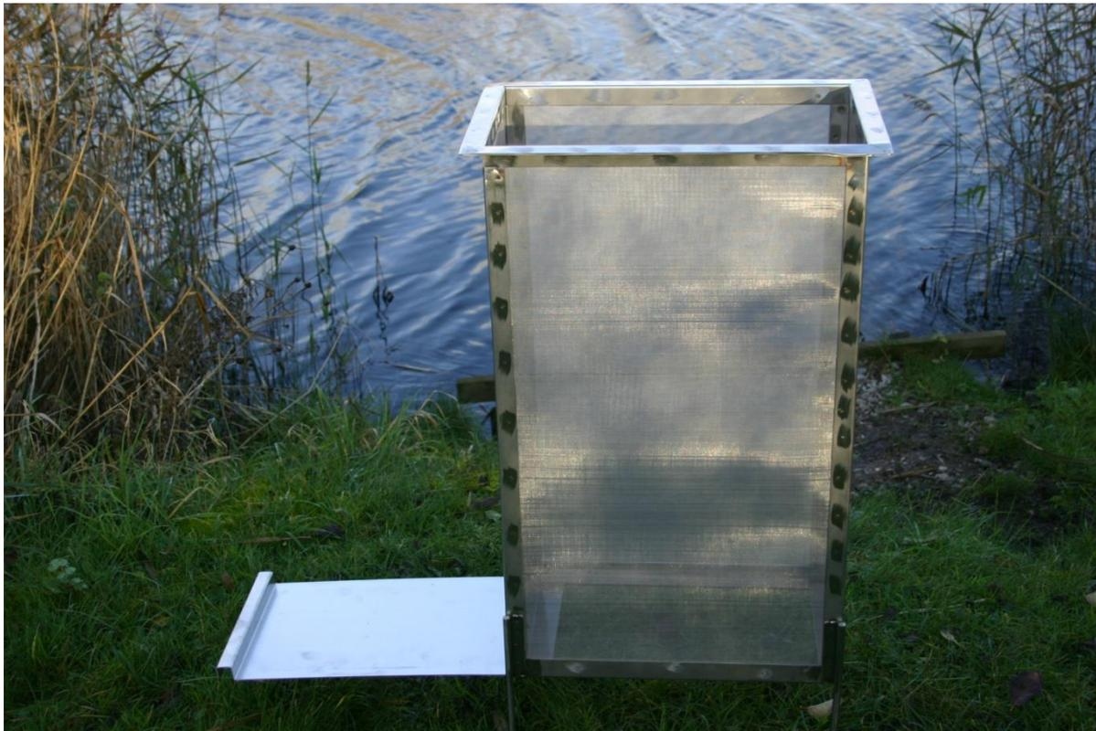
Figure 1 - Modified Gerking box sampler with cutting blade retracted.
