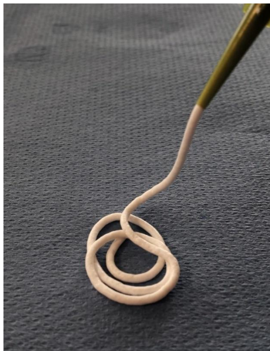
Fig. 3.12. Extrusion of XG-SA-TCP paste through a 1.6 mm nozzle.
