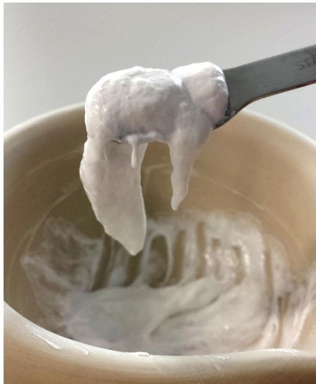
Fig. 3.11. Consistency of XG-based TCP paste (2% w/w and 50% solids).
