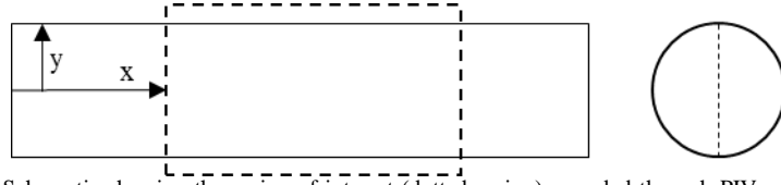
Fig. 4 (Left) Schematic showing the region of interest (dotted region) recorded through PIV experimentation. All analysis was performed at the central longitudinal location. The coordinate system is also provided for reference. (Right) Cross section of the phantom with the dotted line representing the plane used for experimental analysis
