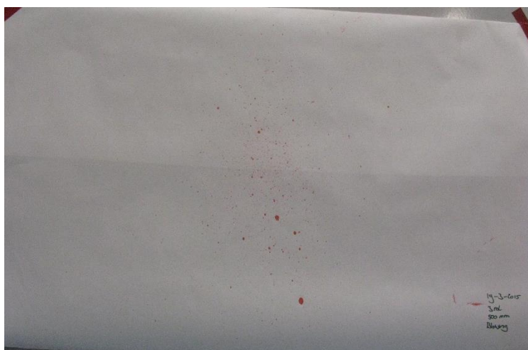
Fig. 11 Pattern on the vertical surface caused by blowing 3 ml of SBS at a 500 mm distance
