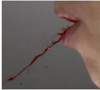
Fig. 8 Coughing 1.5 ml of SBS with an open mouth produced long ligaments which were projected downwards
