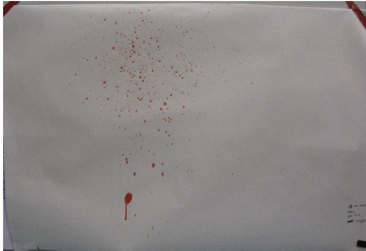
Fig. 12 Pattern on the vertical surface caused by coughing 3 ml of SBS at a 500 mm distance
