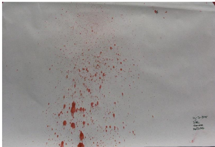
Fig. 13 Pattern on the vertical surface caused by spitting 3 ml of SBS at a 500 mm distance
