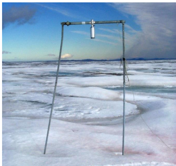
Sonic sounder for snow elevation measurements at AWS site B13 on Brúarjökull, (picture taken by F. Pálsson in September 2001).
