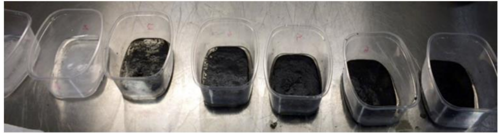
Fig. 4 During the AoI-2015 experiment, different ash concentrations were applied to ice indoors
