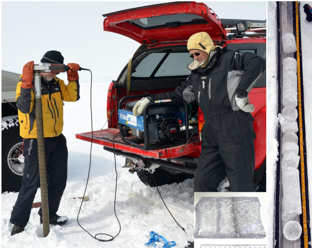
Figure 7: Firm core drilling on Brúarjökull with the Icelandic glaciological Society, Jörfi. On the right pictures: the drilled core, broken into segments with a close up with of sample A20, showing the 2011 dust layer.
