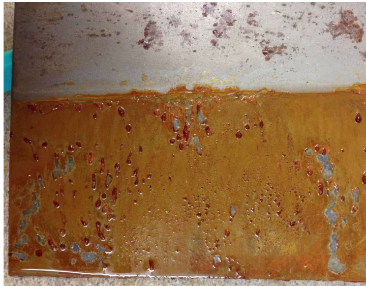
Figure 5-22 – Accelerated Sample with Early Rust Formation
