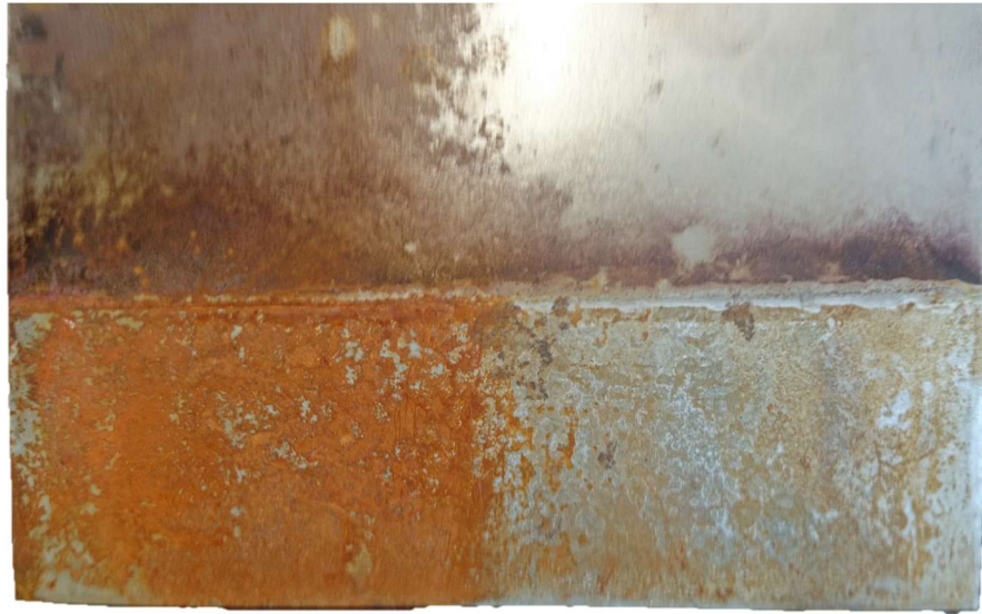
Figure 5-9 – Measurement Areas of Accelerated Ageing on Steel Plate
