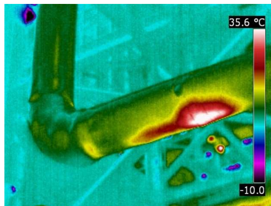
Figure 2-6 – Infrared Image of Pipeline Section [27]
