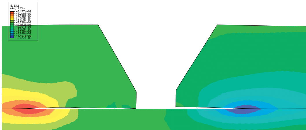
Fig. 19. The shear component of the Cauchy stress at a time of 150.0 \mu\text{s} .
