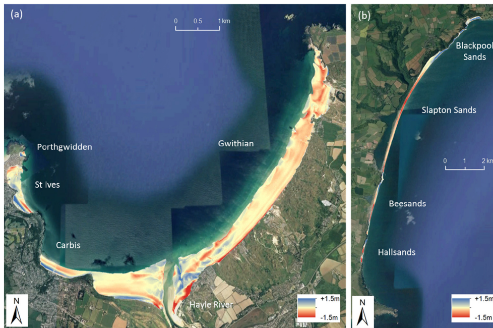
Fig. 13. DoDs obtained from LiDAR data along (a) St. Ives Bay beach surveyed in April 2012 and April 2014, and (b) Start Bay surveyed in April 2012 and April 2014, illustrating spatial change in beach response and sediment connectivity between adjacent beaches at a local scale. Their location along the south west coast of England is presented in Fig. 12. Erosion is coloured in red whereas accretion is coloured in blue. This figure is available in colour online at https://www.journals.elsevier.com/geomorphology . (For interpretation of the references to colour in this figure legend, the reader is referred to the web version of this article.)
