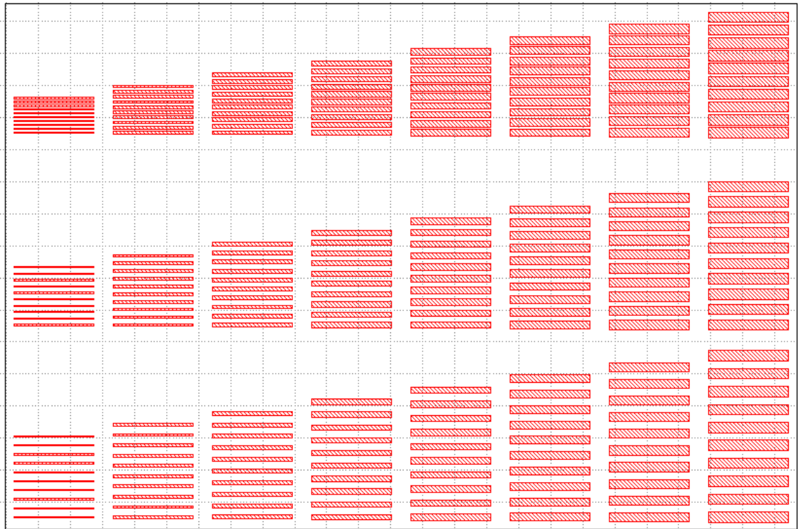
Fig. A.8 Zoomed test vehicles for width and space of horizontal MET1 bars
