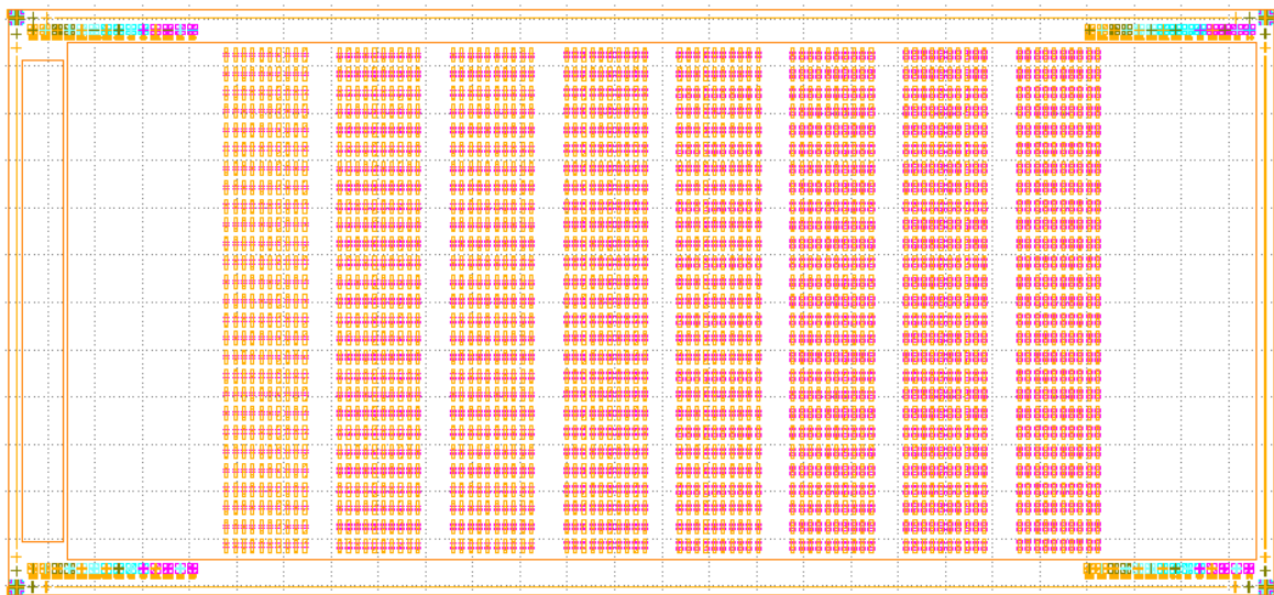
Fig. A.7 Test vehicles for spacing and width of two layers together
