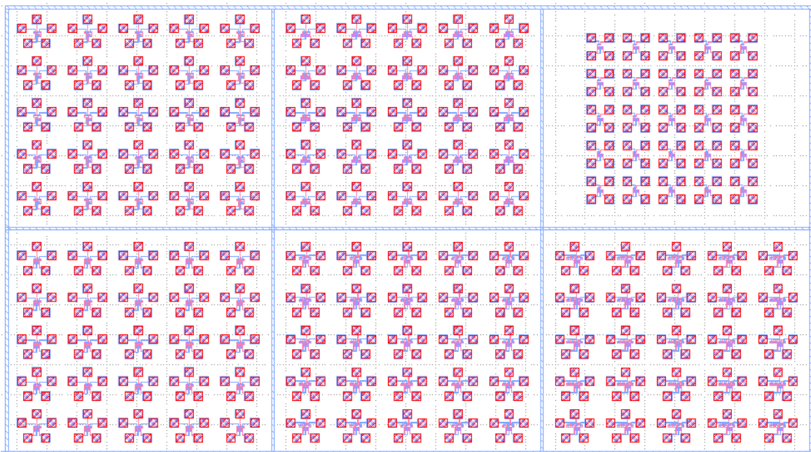
Fig. A.20 Digital logic gates (NAND, NOR, INV) layout
