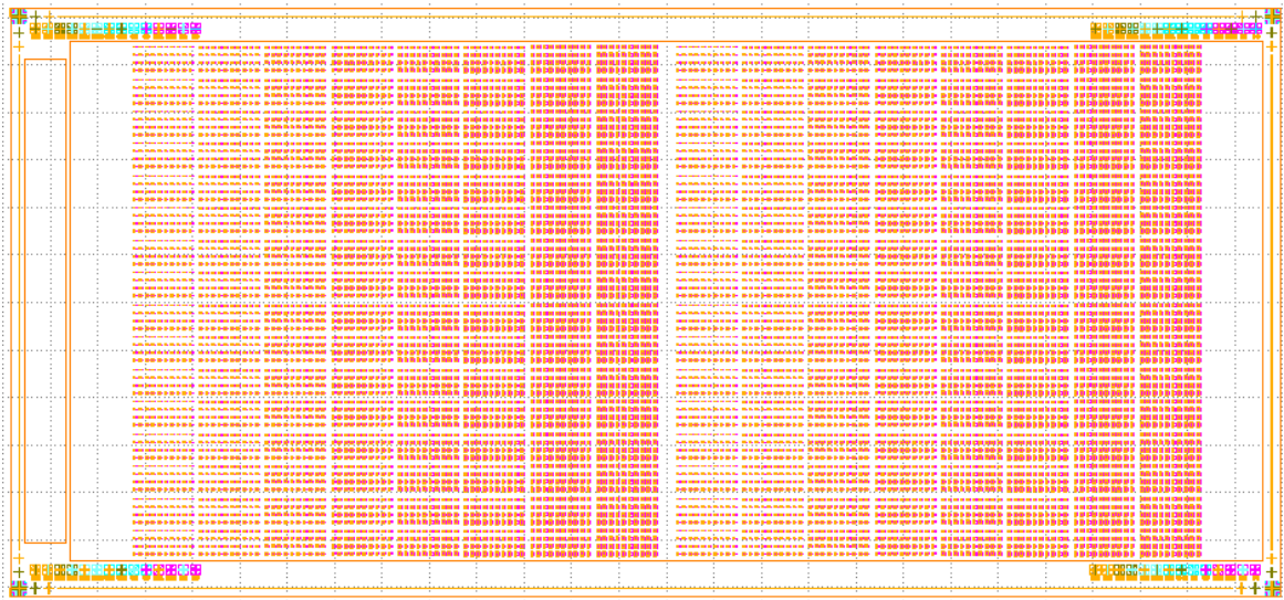
Fig. A.5 Test vehicles for extension, overlap, and width of two layers together (another shape)
