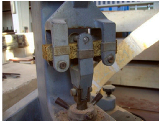
Figure 5. Three-point flexural test performed on a sample.
