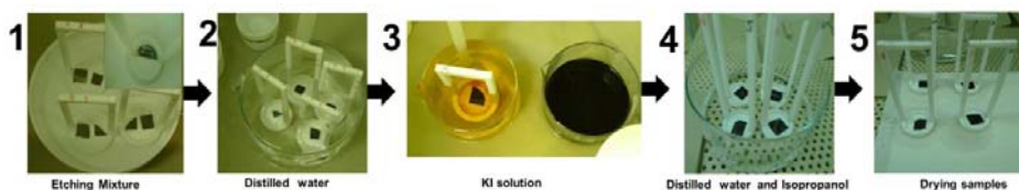
Figure 2.11. Photos describing the procedure of metal-assisted chemical etching to create the Si nanopillars at Clean Room facilities.
