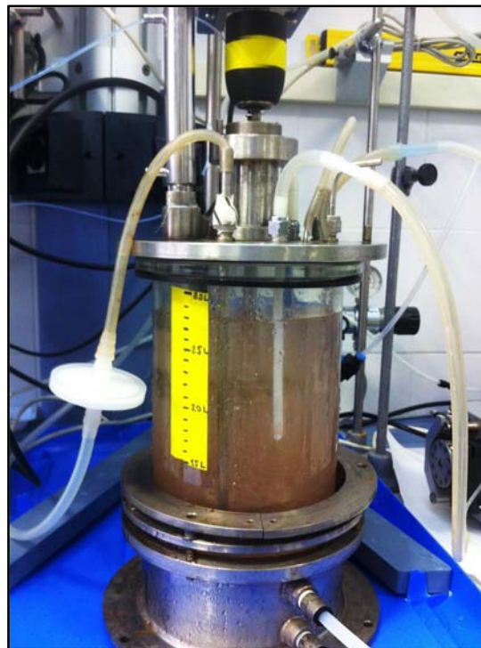
Fig. 5.1. Image of the lab-scale chemostat used for the kinetic experiments.
