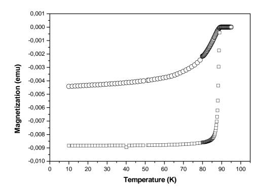
**Figure 6**. Zero-field cooled DC-susceptibility as a function of temperature, showing a  $T_{c,onset} = 89$  K for the YBCO/BZO composite film ( $\circ$ ) and BZO-free YBCO film shown for comparison ( $\square$ ). H= 2 Oe.
