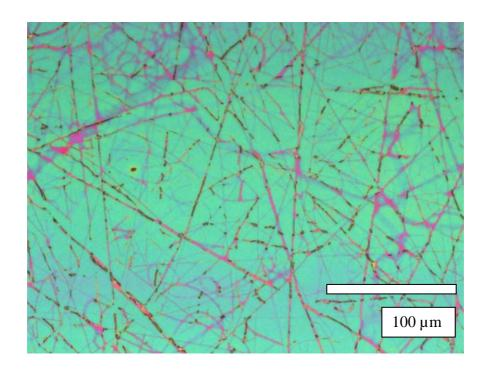
**Figure 2.** Optical image corresponding to the pyrolyzed YBCO-TFA layer with the BZO fiber network, which can be clearly observed.
