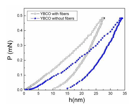
**Figure 7.** Representative load-displacement nanoindentation curves corresponding to the YBCO films with and without the presence of electrospun fibers.
