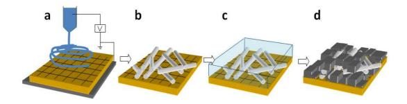
**Figure 1**. a) Electrospinning of BZO precursor fibers on LAO single crystal. b) BZO fiber network after thermal treatment. c) Spin-coating of metalorganic YBCO precursor solution on top of the BZO fiber network. d) Epitaxial film with embedded BZO fibers after the crystal growth of YBCO.
