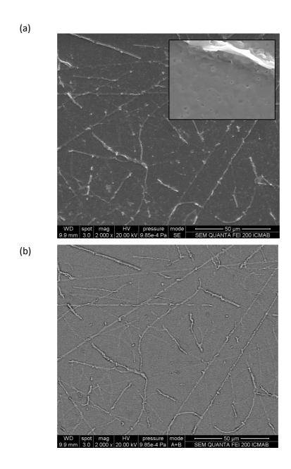
**Figure. 3.** a) Secondary electron FESEM image of the obtained nanocomposite. The BZO fiber network in the YBCO layer can still be observed after the YBCO conversion at high temperature. Inset showing a close-up secondary electron FESEM image showing high density c-axis oriented YBCO region near a BZO fiber. b) Backscattered FESEM image that reveals embedded BZO fibers inside the YBCO epitaxial matrix.
