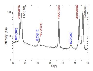
**Figure 5**. a) GADDS frame of the YBCO/BZO fiber and b) integrated  $\theta$ -2 $\theta$  diffraction pattern.
