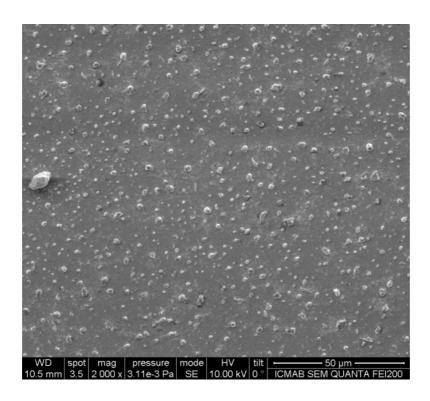
**Figure 4.** FESEM image corresponding to the BZO-free YBCO film prepared for comparison purposes.
