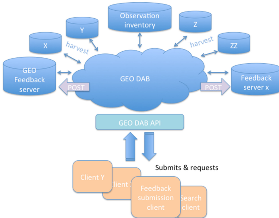
Figure 10: Architecture of GEO DAB connecting with clients, feedback server and the observation inventory.
