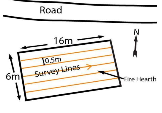
Left, a map of the survey grid. Along the width of the grid, stakes placed 0.5 m apart distinguish profile spacing. Along the length of the grid, GPR measurements were recorded every 0.05 m, utilizing unshielded 400 MHz antennas spaced 0.6 m apart.
