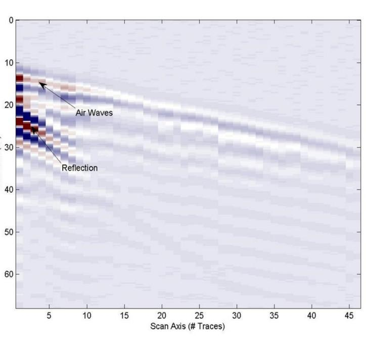
Ξ 0.4 Left, velocity profile created using the common midpoint test. By obtaining a reflection curve from a single horizontal feature, we can model wave velocity through the subsurface.
