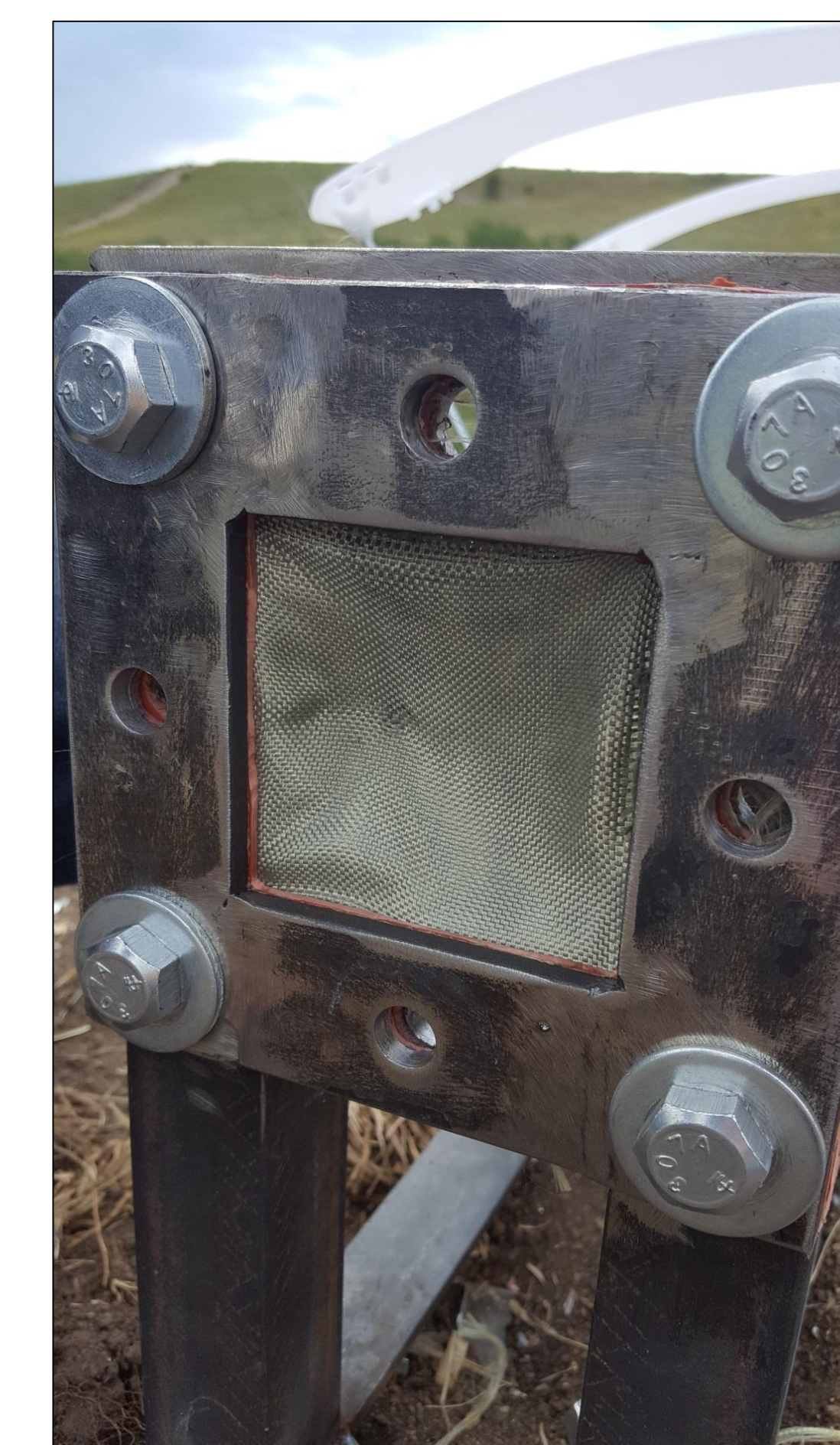
Kevlar after being shot with .177 caliber air rifle still in sample holder. Note: lack of damage to weave
