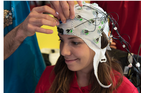
Figure 2: An electroencephalography (EEG) cap.
